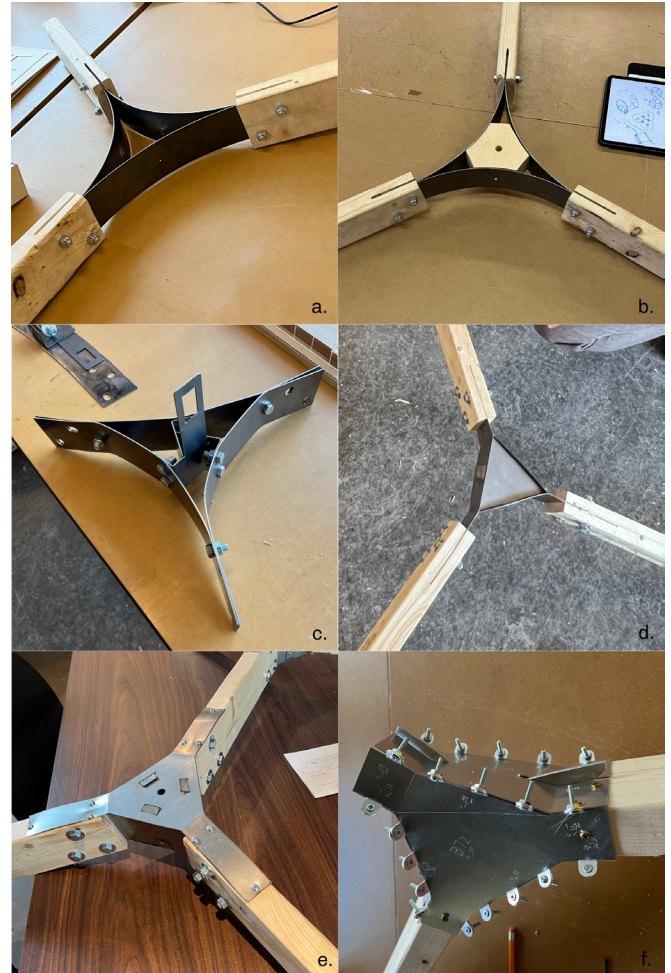
4 Evolution of the node design from curved strips to the augmented shell.
